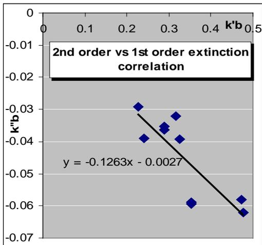
Figure 4: Possible correlation between 1<sup>st</sup> and 2<sup>nd</sup> order extinction
