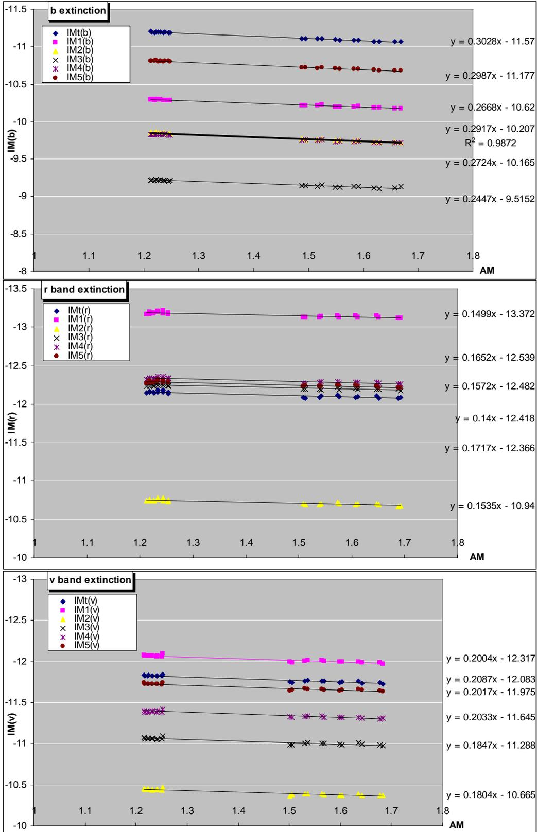
Figure 1: b, r, and v 1<sup>st</sup> order extinction plots for UT 01-18-2005
